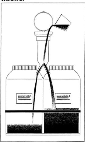
If sample is poured slowly or "dribbled" into device, unequal splitting will occur.
